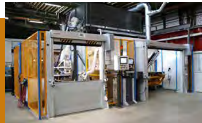
New variants of the VW underride guard are manufactured on a new welding system at the Iserlohn plant. One or two additional base plates reinforce the underride guard for the use of heavier, more powerful batteries for greater range.
