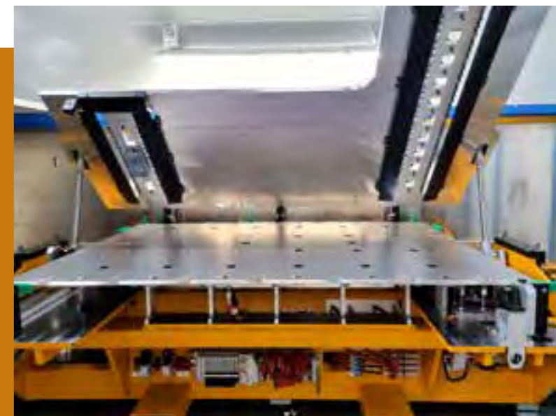
Underride guard in the welding fixture.
